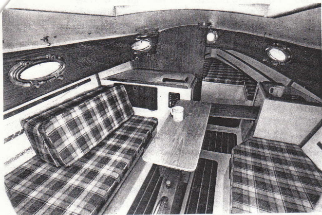
Flexible Interior. Both the table and the bulkhead are removable for more openness below (left), and the insert panel turns the port settee into a double berth.
